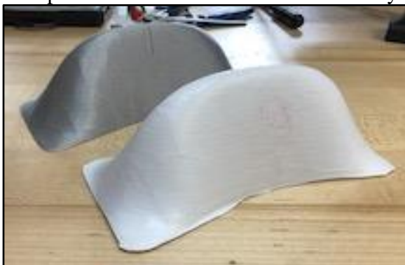
3D printed and vacuum formed rover body
